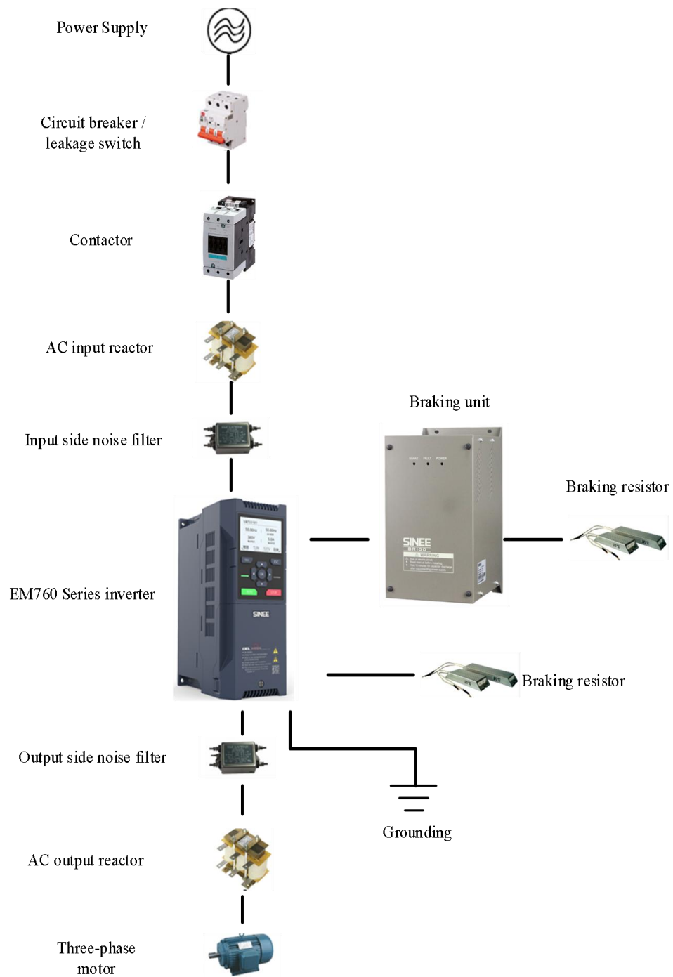
Fig. 3-1 Connection of Inverter and Peripheral Devices
