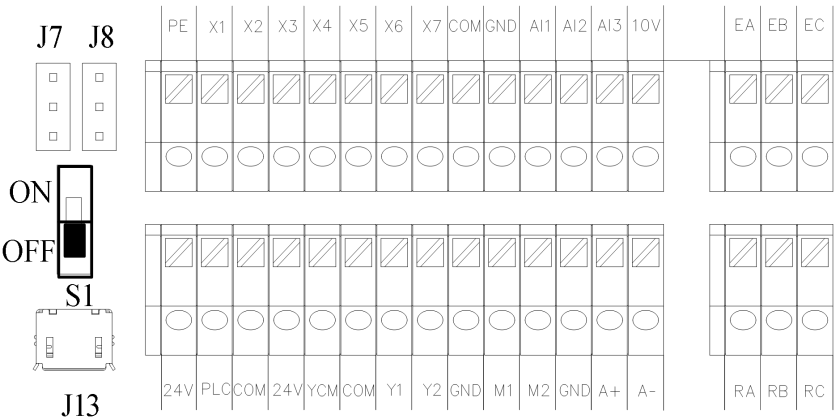
Fig. 3-16 Layout of Control Circuit Terminals
