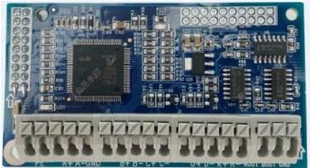
Fig. 9-22 SinCos PG card - real product PG card
