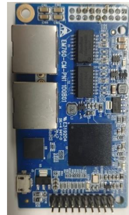
Fig. 9-26 PROFINET communication card - real product
